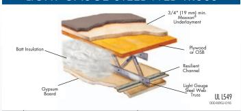
1 HR | w/ Insulation & Resilient Channel | L549, L551, L552, L560
